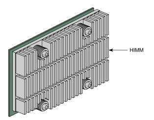
Figure 2-2 Horizontal In-Line Memory Module
