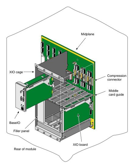
Figure 2-21 Physical Location of the Midplane in Deskside Enclosure
