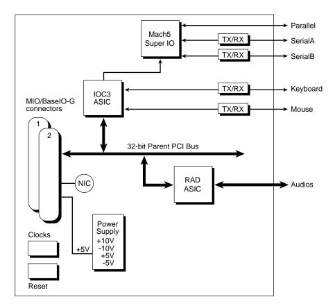
The logical location of an MIO card, connected to an BaseIO-G board, is shown in Figure 2-24. A block diagram of the MIO board is shown in Figure 2-27.
