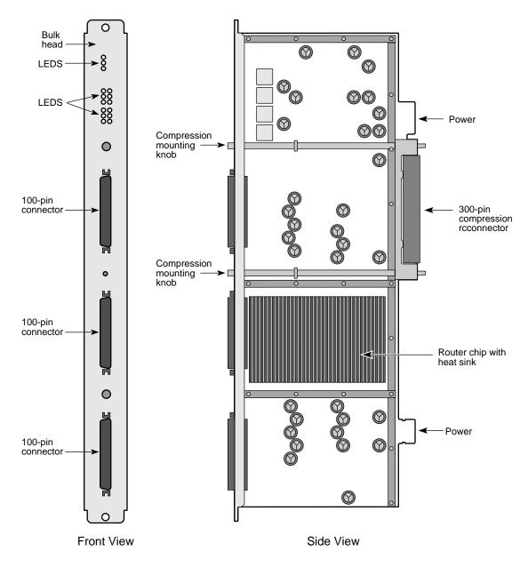
Figure 2-16 Physical View of the Router Board
