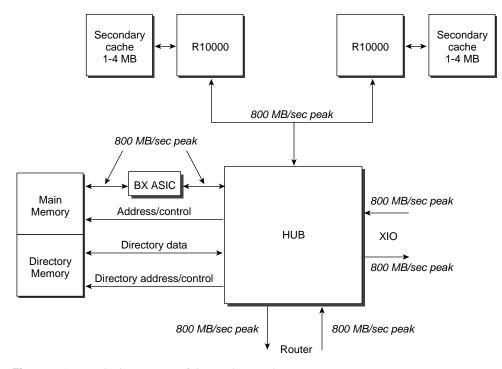
Figure 2-1 Block Diagram of the Node Board
