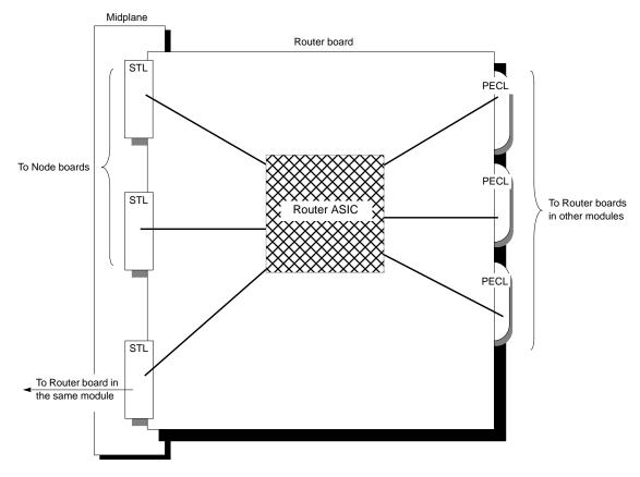
Figure 2-17 Routing Board Connectors
