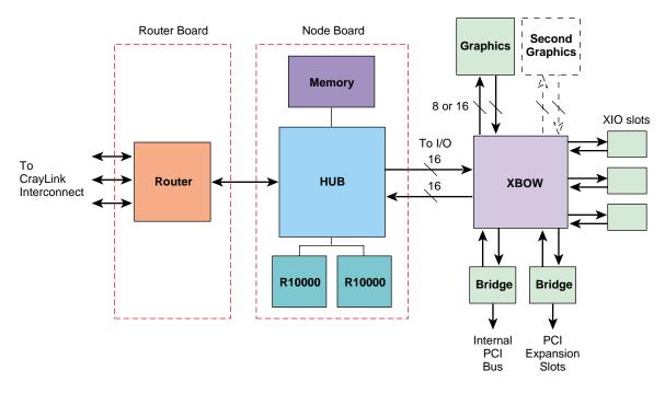
Figure 1-8 Origin2000 Block Diagram
