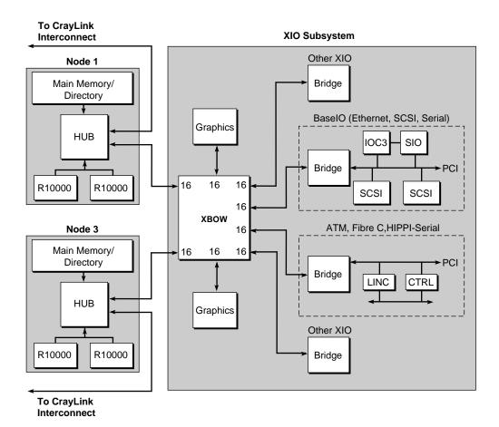
Figure 2-14 Crossbow Connections
