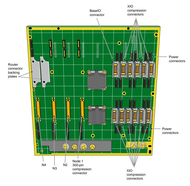
Figure 2-23 Rear View of the Origin2000 Midplane Board
