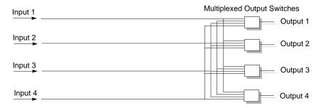
Figure 1-16 Logical Illustration of a Four-by-Four (4 x 4) Crossbar
