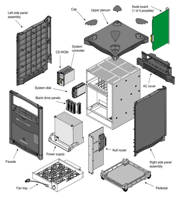
Figure 1-10 Exploded View of the Origin2000 Deskside Chassis
