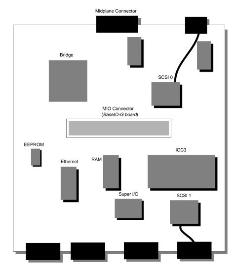
Figure 2-26 Physical Layout of the BaseIO Board
