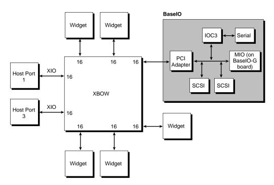
Figure 2-24 Logical Location of an BaseIO Board in an Origin2000 System
