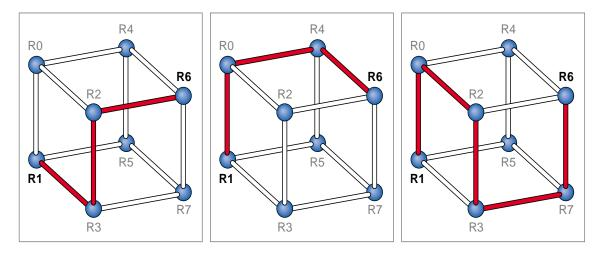
Figure 1-15 Datapaths in an Interconnection Fabric
