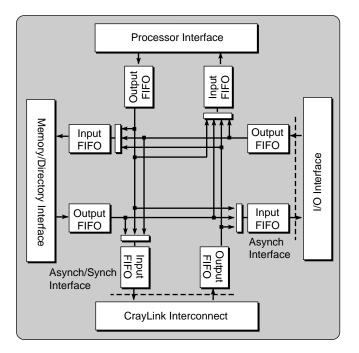
Figure 3-2 Block Diagram of a Hub ASIC
