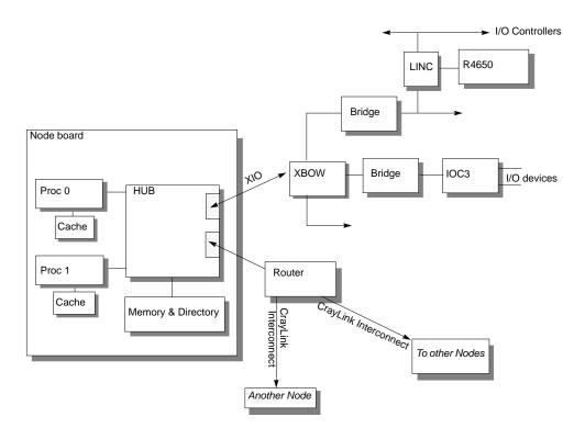
Figure 1-14 Block Diagram of an Origin2000 System
