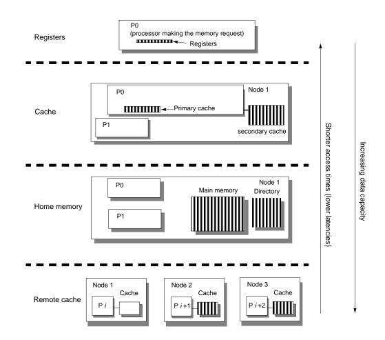
Figure 1-18 Memory Hierarchy, Based on Relative Latencies and Data Capacities
