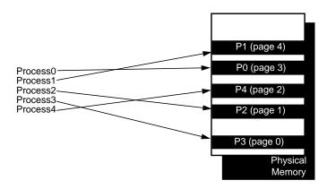
Figure 2-6 Allocating Physical Memory to Virtual Processes
