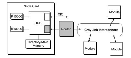
Figure 2-15 Location of a Router Board in an Origin2000 System
