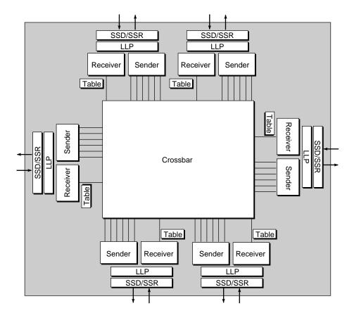
Figure 3-3 Block Diagram of the Router ASIC
