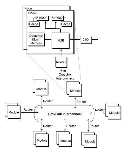
Figure 1-2 Nodes in an Origin2000 System
