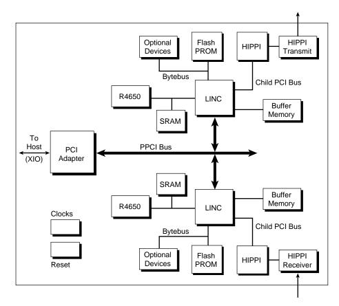
Figure 3-7 Block Diagram of LINC ASICs With Bridge ASIC
