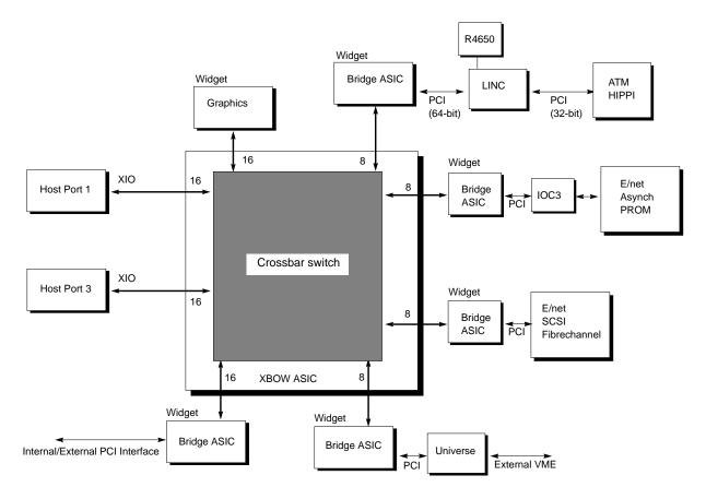
Figure 3-5 Block Diagram of a Crossbow ASIC, Showing Eight Ports Connected to Widgets
