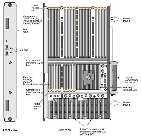
A physical view of the Node board is given in Figure 2-13.
