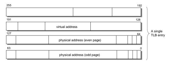
Figure 2-8 Virtual-to-Physical Address Mapping in a TLB Entry
