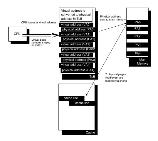
Figure 2-7 Converting Virtual to Physical Addresses
