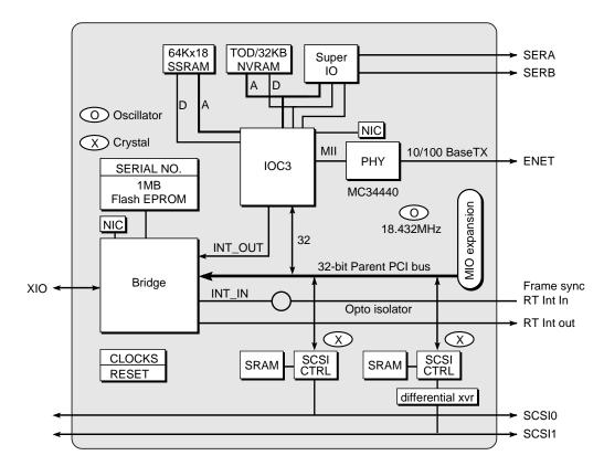
Figure 2-25 BaseIO Board Block Diagram
