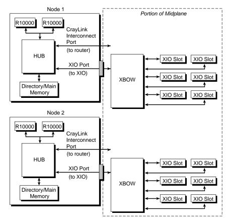
Figure 3-4 Functional Location of Crossbow ASIC
