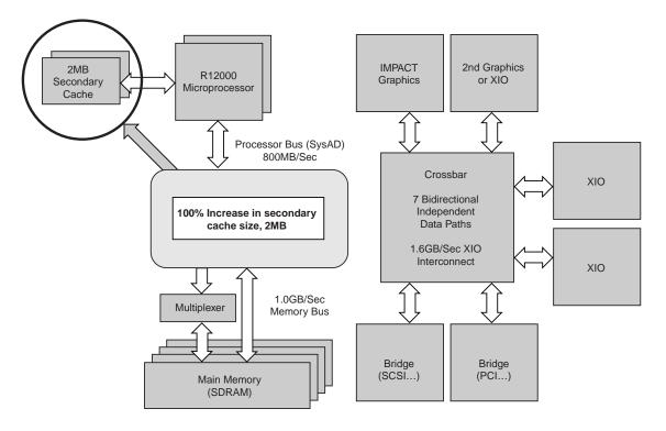
Figure 12. OCTANE System Architectural Changes with MIPS R12000
