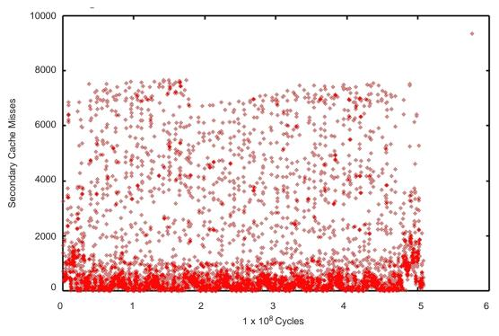
Figure 14b. Observed Secondary Cache Misses Seen on MIPS R12000 During CATIA SolidE Update Test
