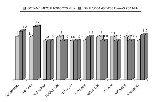
Figure 5. Comparison between Power3 and MIPS R10000 of SPECfp95 to SPECfp\_base95 Results across All Tests
