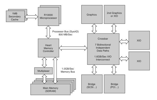
Figure I. OCTANE System Architecture
