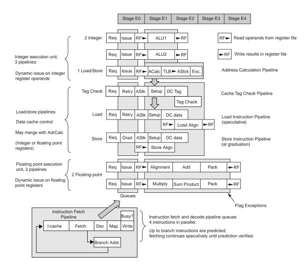
Figure 11b. MIPS R12000 Timing Pipeline
