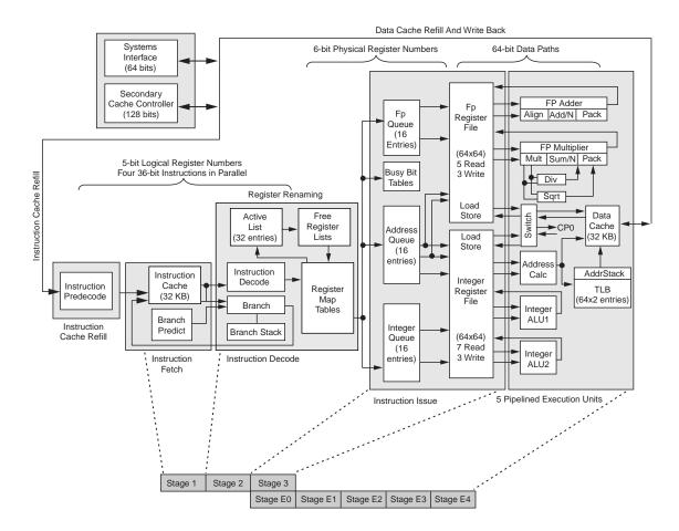
Figure 10a. MIPS R10000 Microprocessor Architecture
