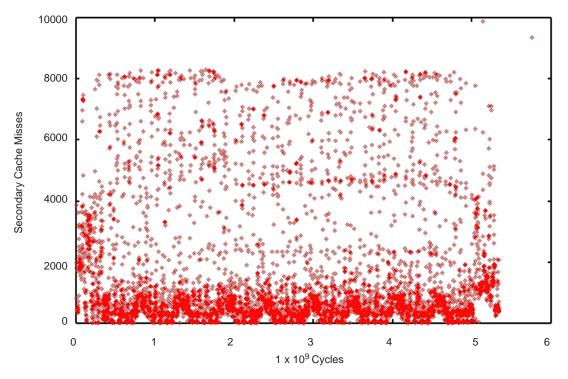
Figure 14a. Observed Secondary Cache Misses Seen on MIPS R10000 During CATIA SolidE Update Test.
