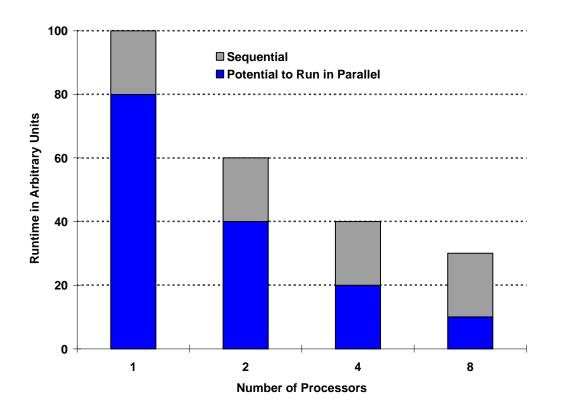
Amdahl's Law is of utmost importance in understanding and gauging parallel performance; thus, included on each of the following parallel speedup graphs is the theoretical performance curve predicted by Amdahl's Law. Large deviations from this curve could indicate performance anomalies.
